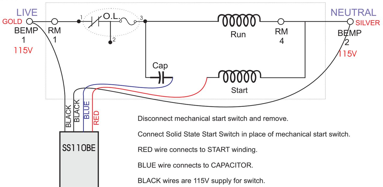
Disconnect mechanical start switch and remove.
