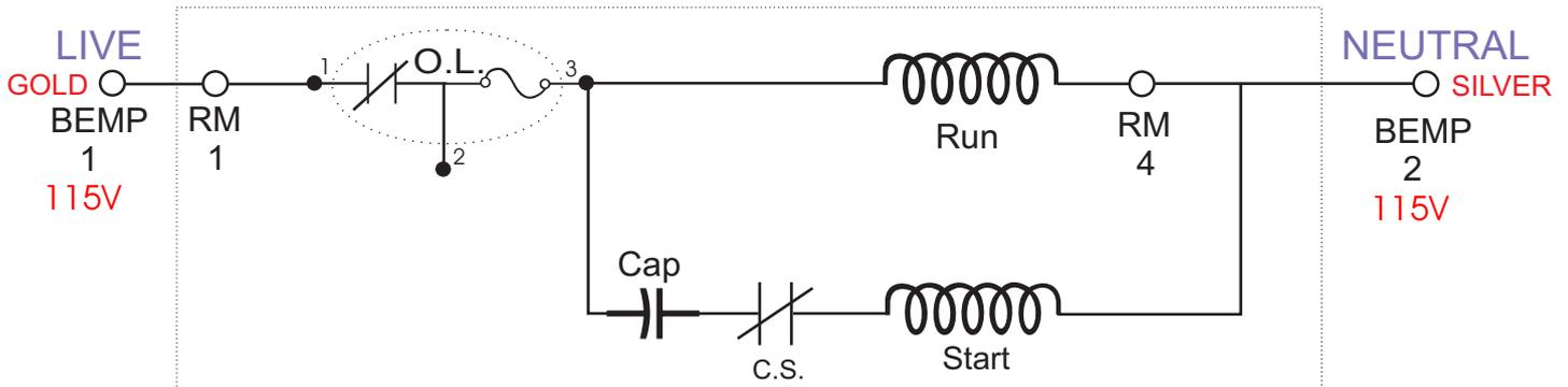
The RED and BLUE wires of the Solid State Start Switch take the place of the mechanical start switch.
